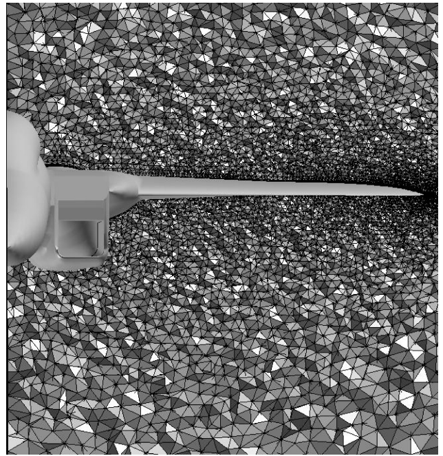
Fig. 2 Baseline computational mesh near aircraft surface.
